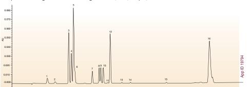
Sample Chromatogram at 280 nm using a Kinetex, C18, 1.7  $\mu m,$  100 x 2.1 mm
